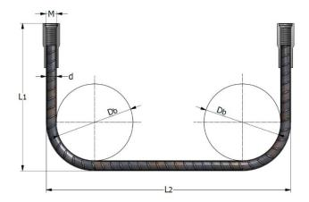
Other lengths are available on request PSAGGD – d x  $L_1x$   $L_2$  in mm
